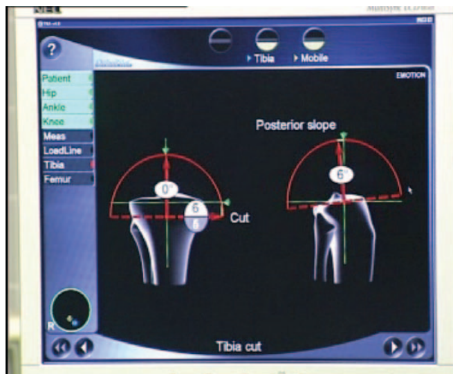
Figure 3 The height of the resection is based on pre-operative planning calculations, its orientation (varus-valgus), and guided and checked on the display.
